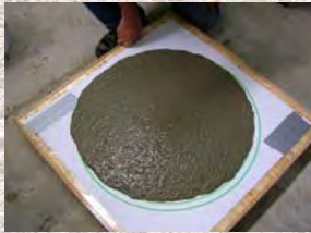
Figure 2.14 Self-consolidating grout specimen.
