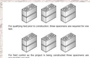
Figure 3.7 Number of specimens for a prism test (ASTM C1314).
