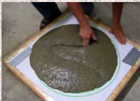
Figure 2.15 Self-consolidating grout specimen - "S" Test.
