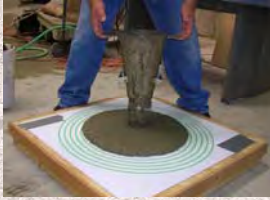
Figure 2.13 Slump flow testing of self-consolidating grout.
